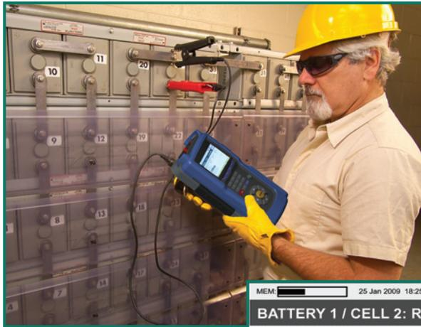
In order to maximize better measurement accuracy and repeatability, the EC1000™ and EC2000™ automatically calculates the proper Battery Calibration Factors (Baselines) during testing. Also, during the battery measurements, measurement limits (Alarms), preset by the user, provide automatic Pass, Warning and Fail visual and audible feedback as to the progress in measuring each cell or block in a battery string.
