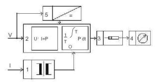
The power converter uses one, two or three for multiplier systems (2) depending on the measurement of balanced or unbalanced load AC systems. Current transformers (1) provide the input current to the multiplier circuit.
