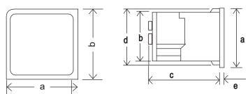
Dimensions WQ 96 WQ 144 (in mm) Bezel 96 144 а 90 136 Case b Depth С 106 106 91.5 137.5 d 5.5 92<sup>+0.8</sup> 5.5 е 138<sup>+1</sup> Cotout Size Depth with 64 64 f ×× . Back cover Weight (approx.) 0.65-0.9 kg. 0.9-1.1 kg.
