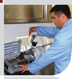
The multifunctional portable test instrument SigmaGT is intended to perform all measurements for testing the electrical safety of portable electrical equipment. The operation of the unit is clear and simple, the operator does not need any special training to operate the instrument. The instrument has a powerful test data management system where auto tests and single tests can be stored in approximately 6000 memory locations.
