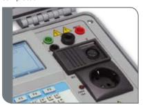
Connector panel - test ports for fixed installed appliances.
