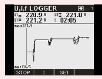
PowerQ Plus enables on-screen evaluation of various pre-set loggers. This is an example of logger for U, I, f.
