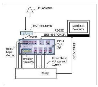
Figure 1: Typical End to End Test Setup
