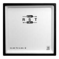
The SQ 0201 phase sequence indicator is intended for determining phase sequences in a three-phase network, from 100 V to 500 V and from 50 Hz to 60 Hz. The indicator is provided with two built-in glow lamps which indicate L1, L2, L3 phase sequence.
