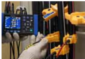
Measure on the outside of cables
