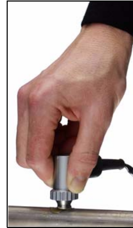
Wall thickness measurement
